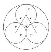
Each side of the equilateral triangle has length 2r. By properties of 30-60-90 triangles, each median of this triangle has length  $r\sqrt{3}$ . Because the centroid of the triangle divides each median in a 2:1 ratio, we have  $R-r=\frac{2}{3}r\sqrt{3}$ . Clearing fractions gives  $3R-3r=2r\sqrt{3}$ . Solving for r gives
